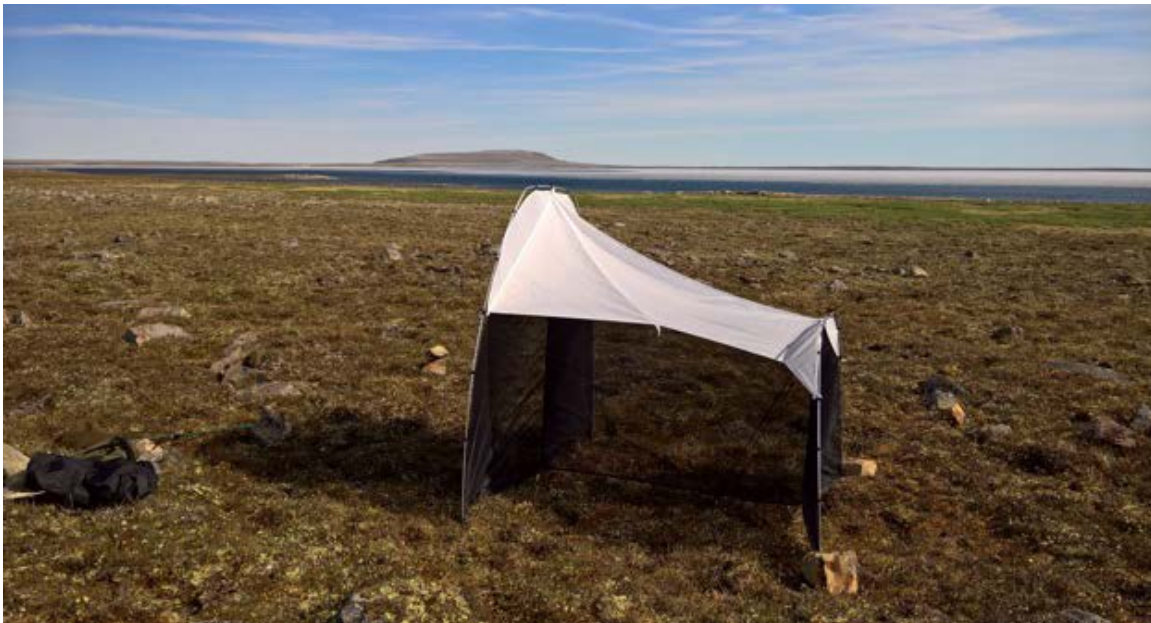
Figure 40. A Malaise trap deployed on the tundra in Nunavut, Canada for biomonitoring arthropods as part of the Arctic BIOSCAN project.
