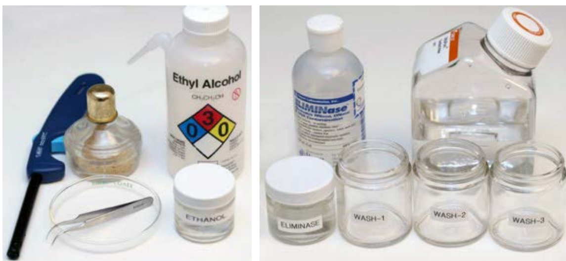
Figure 17. Options for sterilizing forceps/blades after handling each sample. Left: most common setup using a gas burner and ethanol. Right: chemical sterilization using ELIMINase.
