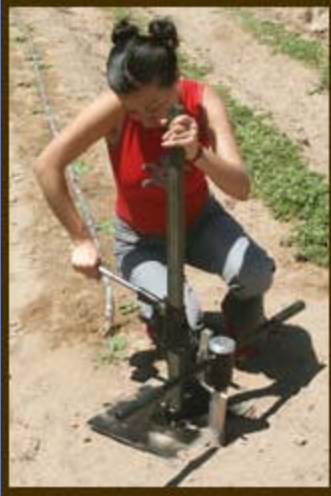
Using the car jack, the soil sampler is easily retrieved in about 2 minutes
