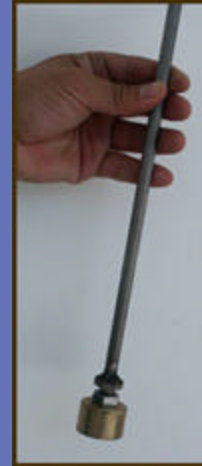
A compactor to help extract the soil core from within the soil sampler and maintain the integrity of the core in light soils
