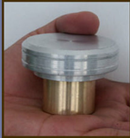
Soft aluminum cap to protect the vertical sampler from the blows from the heavy hammer
