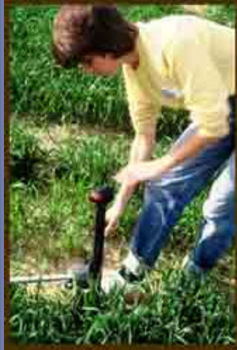
Using the car jack, the soil sampler is easily retrieved in about 2 minutes. Strong workers are not required
