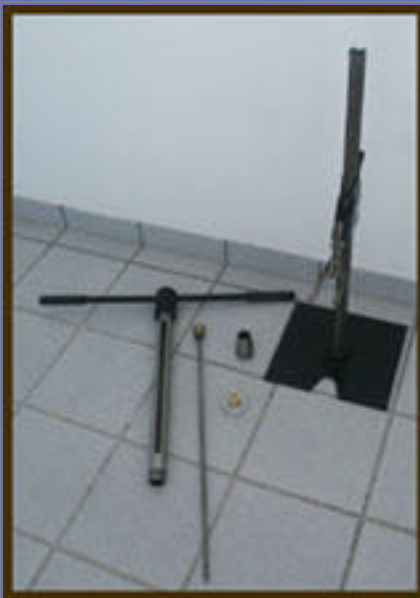
Dismantled assembly for vertical soil core sampler with all necessary parts
