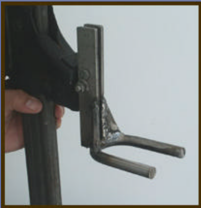
A U-shape jaw accessory mounted on the car jack built to fit the cutting head of the soil sampler. This allows easy lifting of the sampler from the soil.
