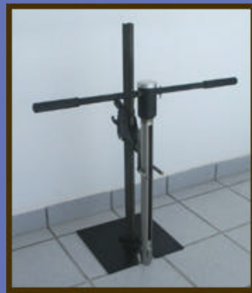
Mounted vertical soil core sampler with all the pieces assembled in their correct position.
