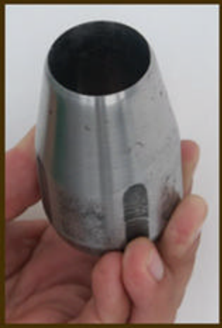
Harden steel cutting head of the vertical soil core sampler screwed to the tube of the sampler by rough threads
